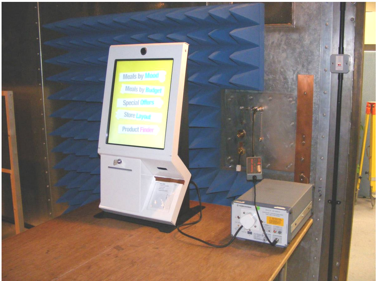
Pic 1. EUT positioned in RF Shielded Enclosure – Conducted Emissions Measurement
