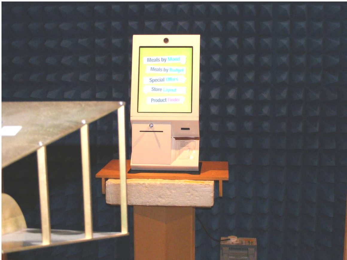
Pic 3. EUT positioned in RF Shielded Enclosure
