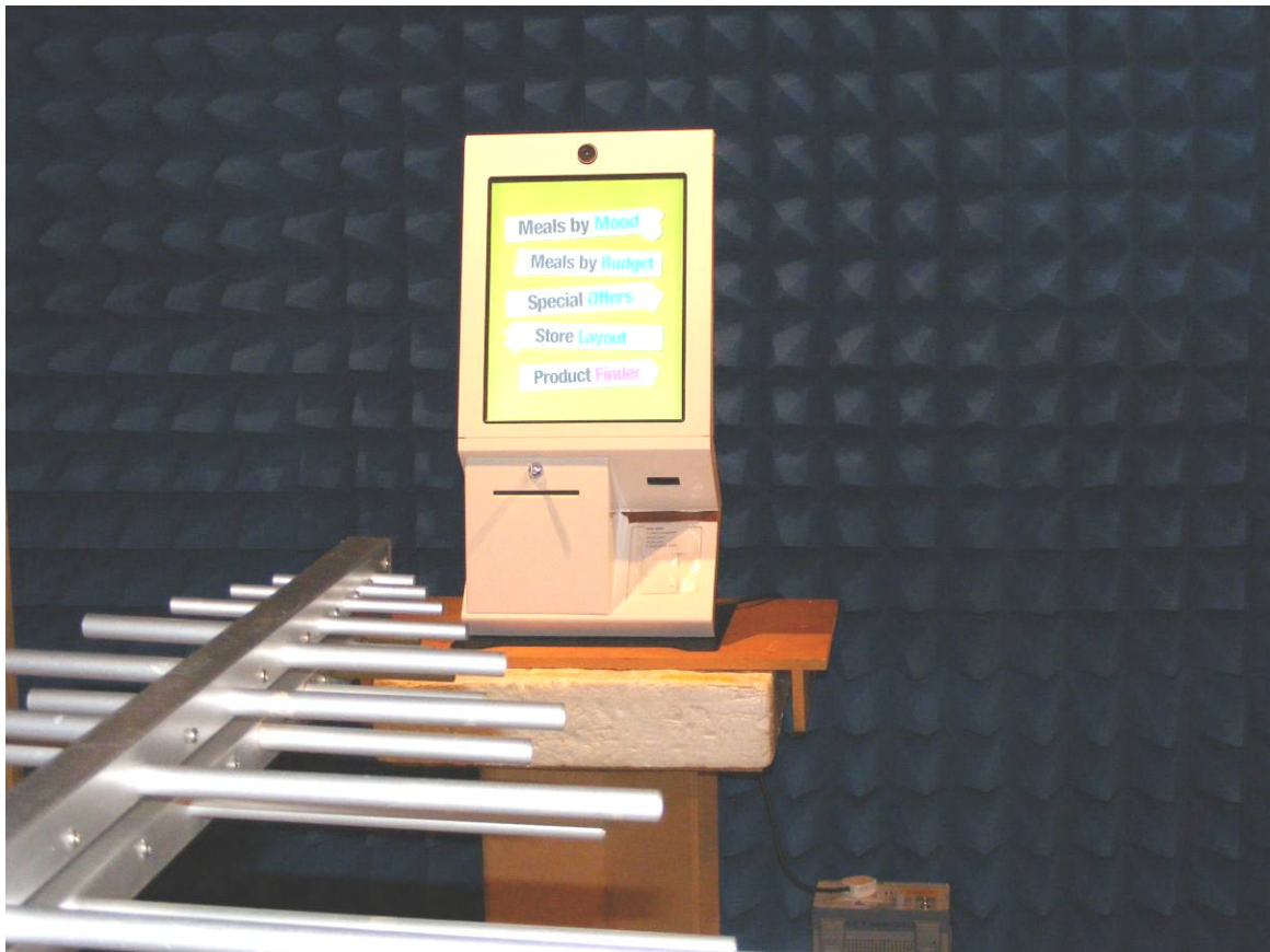
Pic 2. EUT positioned in RF Shielded Enclosure
